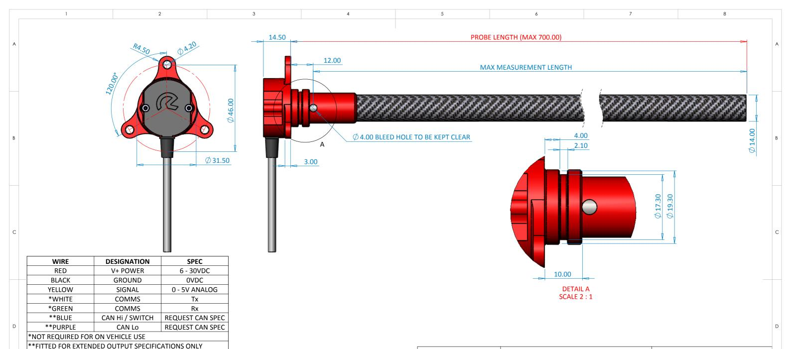
SENSOR TO BE SUPPLIED TO CUSTOMER SPECIFIED LENGTHS, PLEASE CONTACT REVENTEC FOR SENSORS ABOVE 700mm ALL UNITS ARE CALIBRATED AT THE FACTORY IN CUSTOMER SPECIFIED FLUID TO ENSURE OPTIMUM PERFORMANCE. ENSURE SENSOR IS KEPT MINIMUM OF 3MM FROM THE BASE OF THE TANK.
