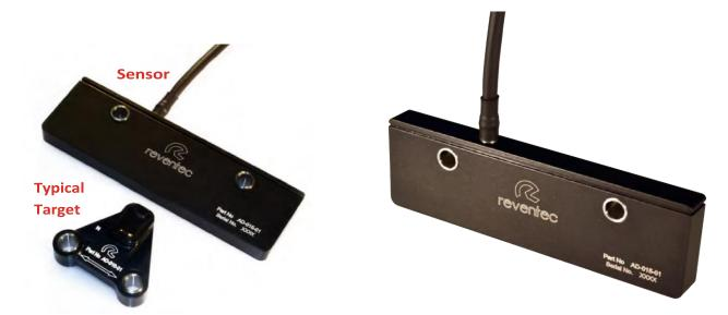
The Quantum100<sup>™</sup> sensor is a robust, lightweight linear position sensor with a 100mm measurement range. The non-contact TMR sensor provides extremely accurate position measurement in harsh environmental applications. Standard motorsport measurement applications include: hydraulic piston travel, suspension component monitoring, steering position and throttle position sensing. The sensor outputs its measurement via a digital CAN output or analogue voltage output.
