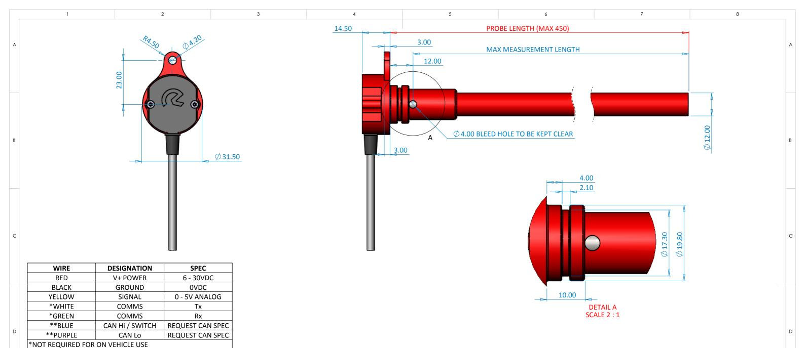
SENSOR TO BE SUPPLIED TO CUSTOMER SPECIFIED LENGTHS, PLEASE CONTACT REVENTEC FOR SENSORS ABOVE 450mm ALL UNITS ARE CALIBRATED AT THE FACTORY IN CUSTOMER SPECIFIED FLUID TO ENSURE OPTIMUM PERFORMANCE. ENSURE SENSOR IS KEPT MINIMUM OF 3MM FROM THE BASE OF THE TANK.
