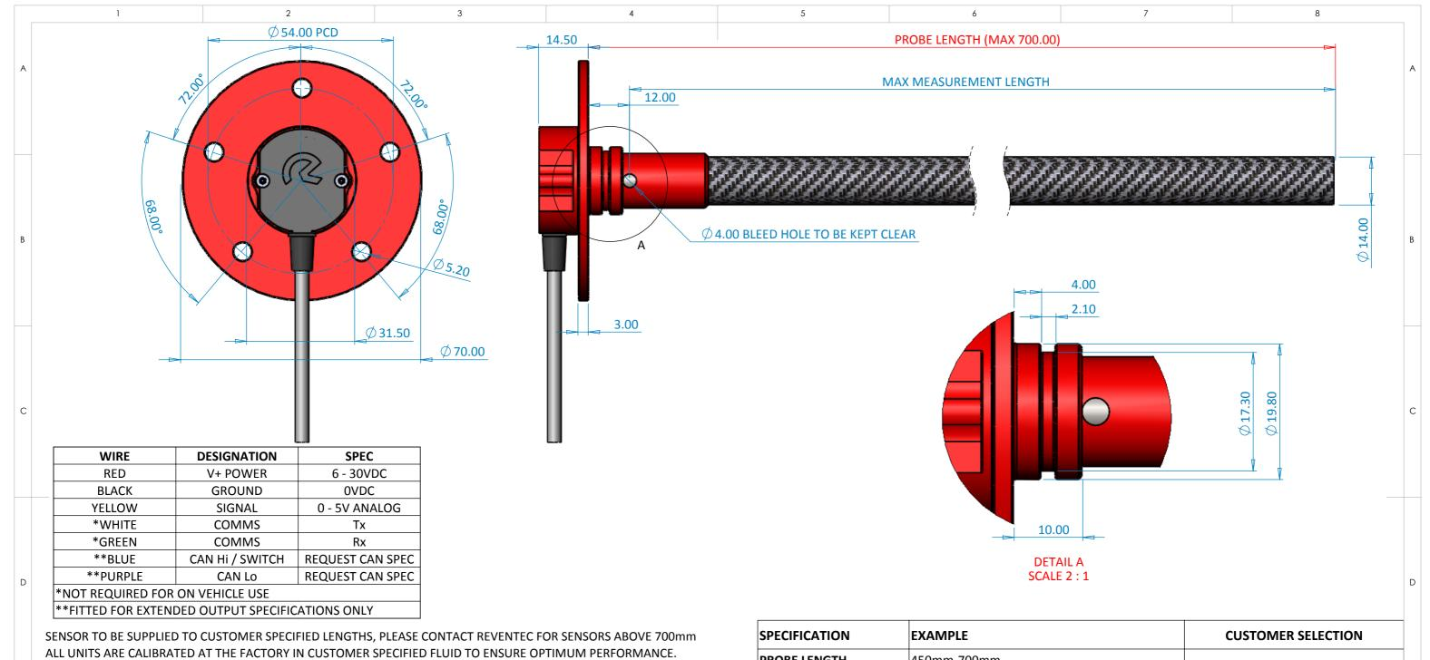
ENSURE SENSOR IS KEPT MINIMUM OF 3MM FROM THE BASE OF THE TANK.
